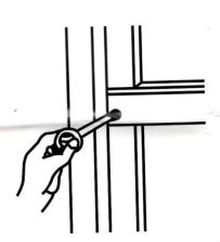
**4.** Close and latch window. Screw Security Screw into window with special key provided.
