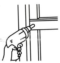
**1.** With the window fully closed AND LATCHED, drill a 11mm (7/16") diameter hole in cross member of inner window through to cross member of outer window to depth of 65mm (2 9/16").
