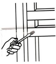
3. Raise inner and lower outer window to allow fitting of small bush to hole drilled in outer window.
